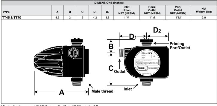
\* Suction & delivery accept  $1^{1/_{2}}$ " PVC pipe on the I.D. and 2" fitting on the O.D.
